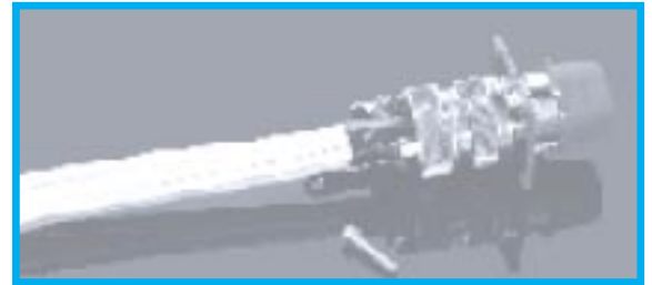
FIGURE 3: Individual Shield Adapter Body assembled to connector, Friction Ring and Nut tightened on Adapter Body with Shield Pigtaills dressed behind the adapter.
